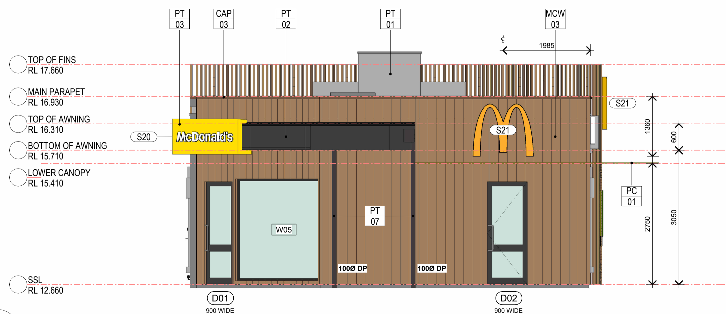
2 BUILDING EAST ELEVATION 1 : 50
